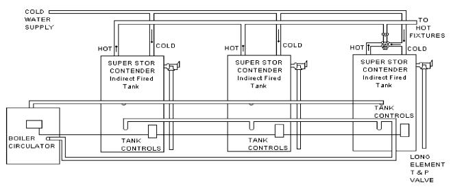
NOTE: ALL PIPING IN PARALLEL IS USED FOR LARGE DUMPS OF HOT WATER; HIGH USAGE, SHORT DURATION.
