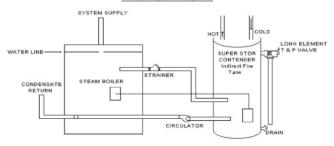
NOTE: WATER LINE MUST REMAIN ABOVE BOILER OUTLET TO WATER HEATER AT ALL TIMES.
