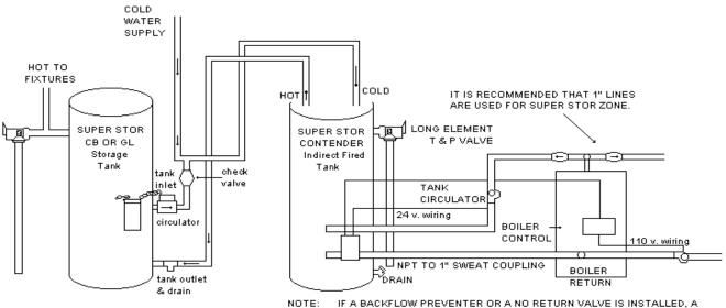
IF A BACKFLOW PREVENTER OR A NO RETURN VALVE IS INSTALLED, A THERMAL EXPANSION TANK IS REQUIRED ON THE COLD WATER INLET BETWEEN THE SUPER STOR AND THE BACKFLOW PREVENTER.
