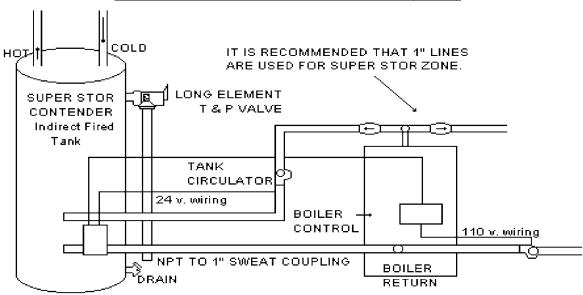
NOTE: IF A BACKFLOW PREVENTER OR A NO RETURN VALVE IS INSTALLED, A THERMAL EXPANSION TANK IS REQUIRED ON THE COLD WATER INLET BETWEEN THE SUPER STOR AND THE BACKFLOW PREVENTER.
